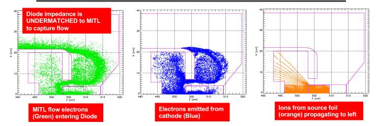
•Prediction of (LEFT) MITL flow into diode, (MIDDLE) emitted electrons from cathode, and (RIGHT) ions in the forward direction. Estimated load voltage is 13-15 MV, due to impedance undermatch).
