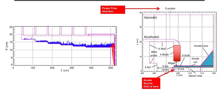
•(LEFT) Simplified drawing of HERMES MITL power flow in negative polarity operation
